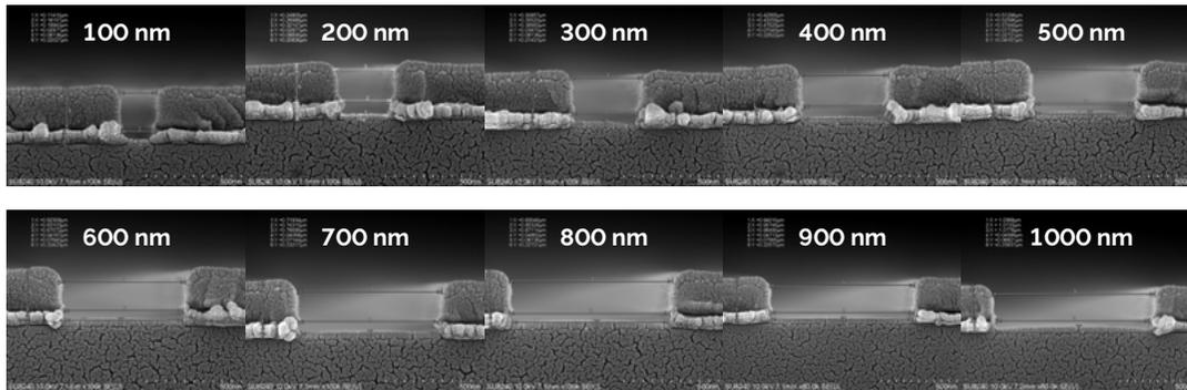
Figure 1: Profile Post Etch of Al with  $\text{Cl}_2/ \text{HBr}/ \text{BCl}_3$ . Very high selectivity to ZEP mask. Al etch profile circa  $> 88^\circ$ . Courtesy of Dr James Grant, Senior Plasma Process Research Engineer in James Watt Nanofabrication Centre.
