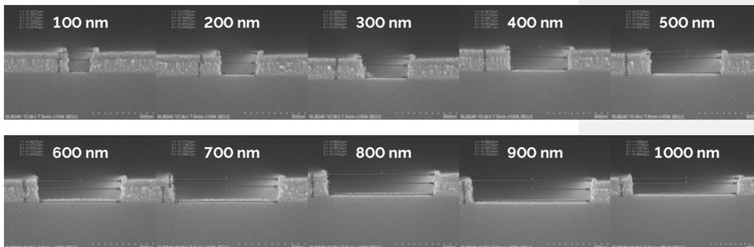
Figure 2: Profile Post Etch of NbN with  $\text{CF}_4$  Ar RIE (ZEP mask still on). NbN etch profile circa  $> 88^\circ$ . Courtesy of Dr James Grant, Senior Plasma Process Research Engineer in James Watt Nanofabrication Centre.
